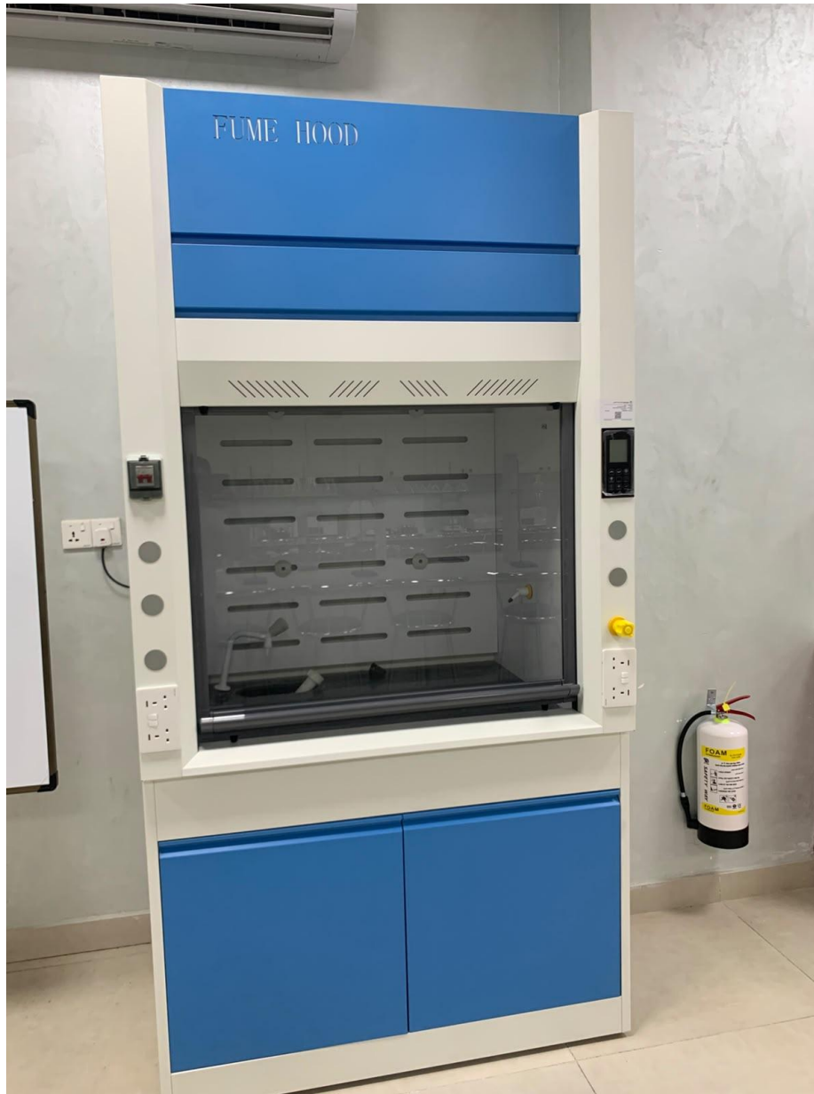
Figure 9.3: Front view of the Fume Hood cabinet showing digital ventilation control panel and sash glass.
