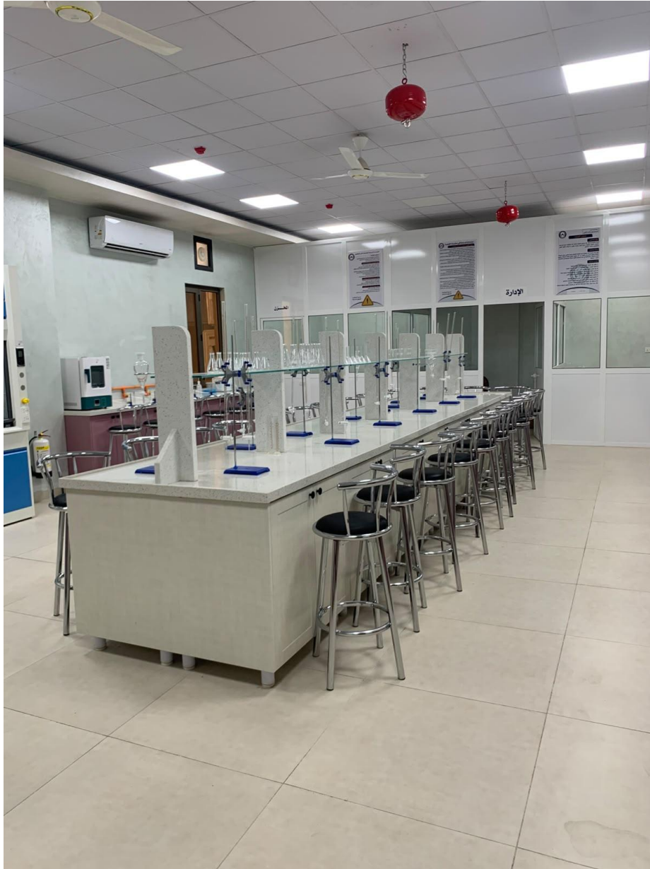
Figure 9.2: Central lab bench equipped with glass reagent racks, burette stands, and ergonomic stainless steel stools.
