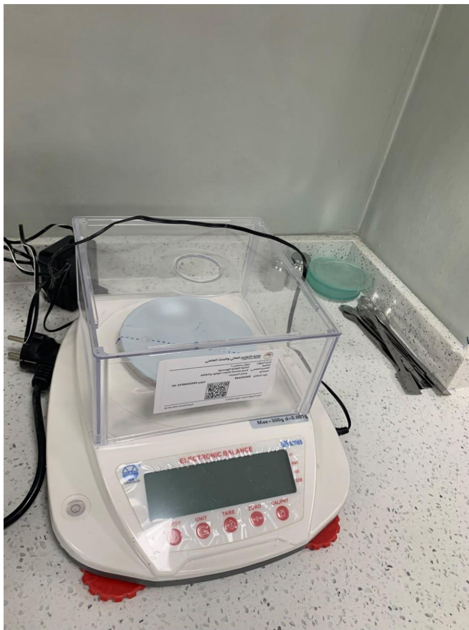
Figure 9.4: Analytical Precision Electronic Balance (0.001g) with glass draft shield and official Ministry Tag.
