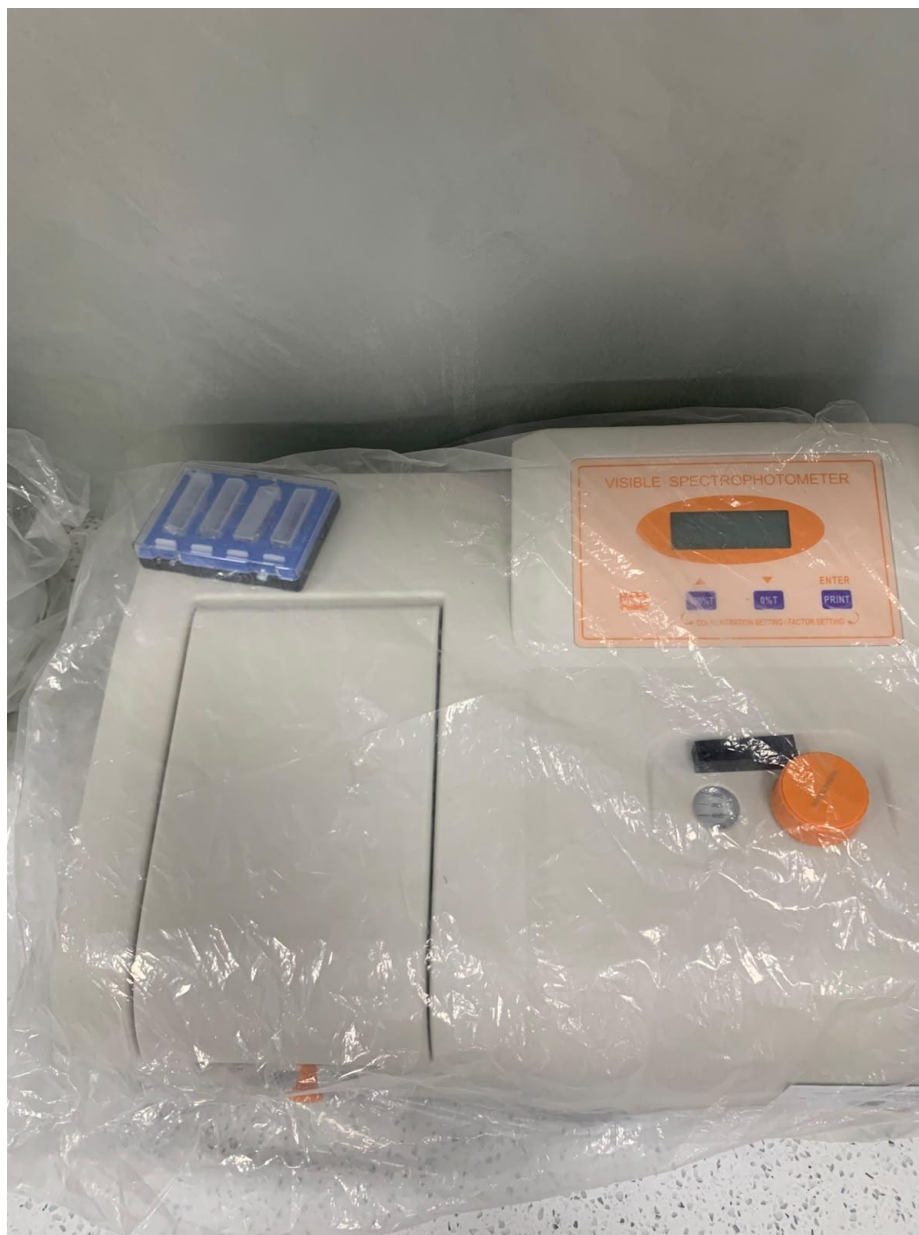
Figure 9.5: Visible Spectrophotometer instrument used for quantitative chemical concentration analysis.
